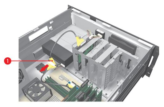
Figure 7. Removing the IDE Data Cable
